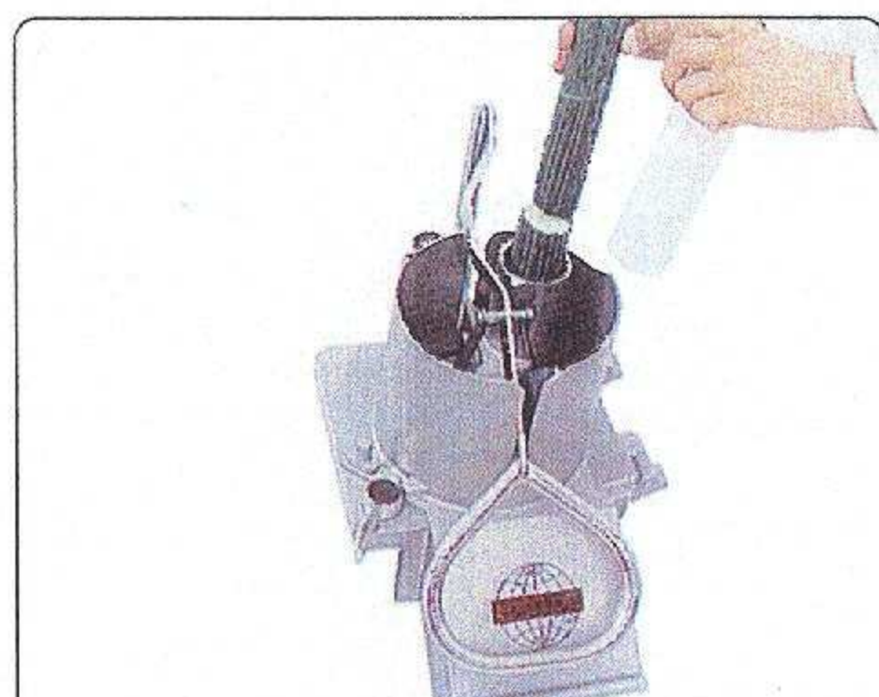
Continuous profile cutting of cucumber, leek, etc.
