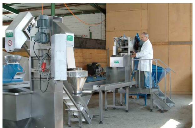
DORNOW peeling machine 20 K-HB / 20 M-HB, manually operated. (Art.-Nos. 0001 und 0020). Industrial construction. Subsequent integration into automatic system possible.
