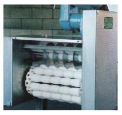
Potato halving machine KT2. You see the circular blades. This machine can only potatoes into two pieces. It does not allow quartering.
