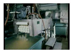
The potato halving and quartering machine KT1E in operation
