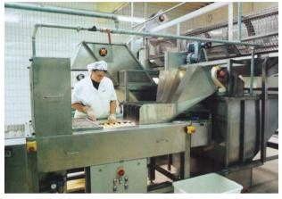
DORNOW potato dividing machine KT1E. This machine can cut potatoes into quarters and/or halves. Right at the top of the picture you see a sorting drum preconnected for peeled potatoes. Right below the potato separating device VE-4R, which feeds the potatoes onto the cutting machine in a steady flow. The above mentioned dividing machine can be used for both halving and quartering.
