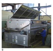
Available in nearly all sizes: screw diameters from 500-2500, roller diameters 100 and 150, roller lengths 2000-4000 mm
