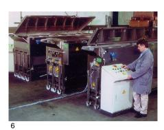
Available in three sizes, can be rapidly converted. Available with blade, carborundum, onion-peeling and special peeling discs
