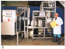
The machines can be supplied with blade, carborundum, onion-peeling and/or special peeling discs for conversion purposes
