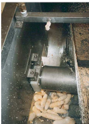
4 • Cassava (manioc) peeling. View inside a DORNOW roller peeler
