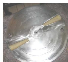
Blade, carborundum and onion-peeling discs for batch peeler type "20"
