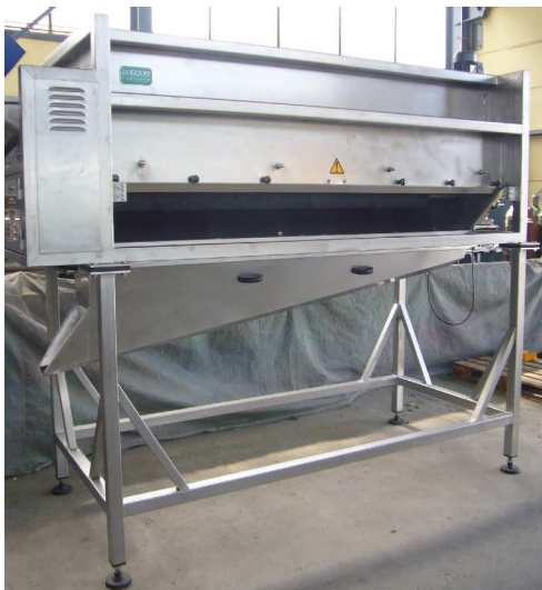
2 • Smallest DORNOW roller peeler R-OW-500-B, 4 rollers, screw conveyor diameter 500, roller length 2000 mm.
