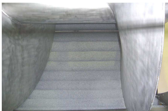
View inside roller peeler R-OW-190-A1, 14 rollers, diameter 150, screw diameter 1900, roller peeler 4000 mm.
