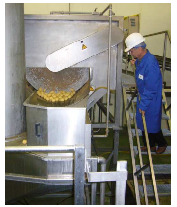
7 • DORNOW roller peeler R-OW-130-A in an industrial potato peeling plant
