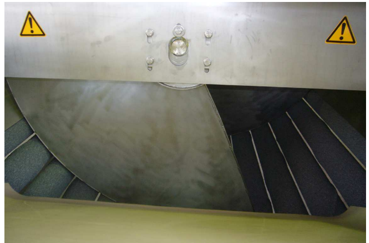
1 • DORNOW roller peeler R-OW-190-A1 in a potato-processing plant. Screw diameter 1900, 14 rollers, diameter 150, roller length 4000 mm, for major industrial use
