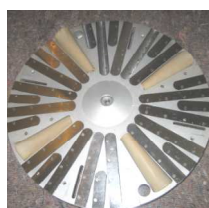
Blade, carborundum and onion-peeling discs for batch peeler type "20"
