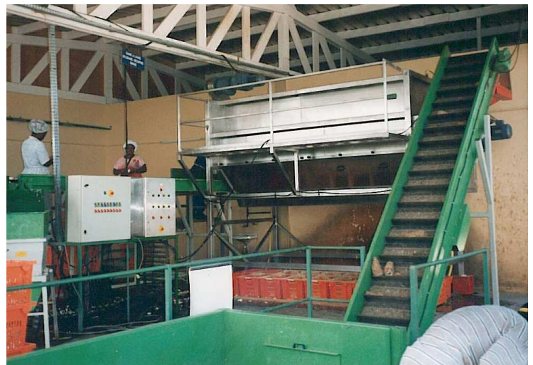
3 • Cassava (manioc) peeling system with DORNOW roller peeler in Africa (R-OW-110-A)
