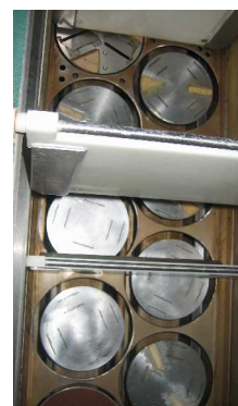
MSS peeling line with onion-peeling discs
