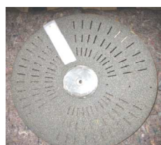
Blade, carborundum and onion-peeling discs for batch peeler type "20"
