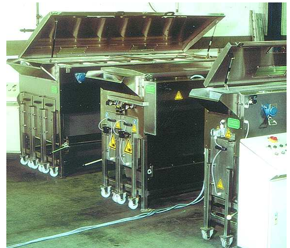
8 • The MSS machines come in 3 sizes: MSS-A with one, MSS-B with two and MSS-C with three peeling lines, can be fitted with blade, carborundum, onion-peeling and various special discs.
