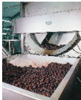
6 • In DORNOW roller peelers, beetroot (cooked and raw) can be peeled with excellent results
