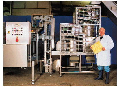
15 • The system is available as an onion-peeling system and/or potato-peeling system with carborundum/blade peeling. Also available in a version that can be converted into a potato-peeling system.
