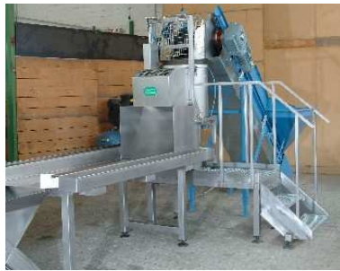
14 • Smaller potato-peeling plant, automatic; quick conversion into onion-peeling plant possible.
