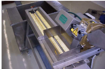
17 • French-fry cutting machine Super XA with sorting equipment 4M.
