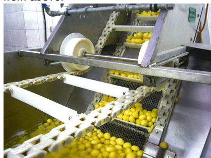
8 • Storage bin behind MSS machine. Functions: storage, washing, dosing.
