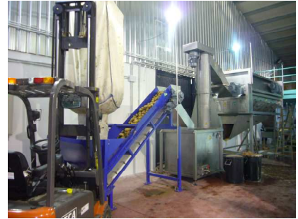
12 • View inside a potato-peeling firm: raw produce in "big bags", dosing belt, stone catcher, roller peeler.
