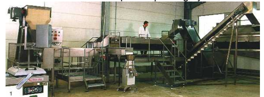
15 • The system is available as an onion-peeling system and/or potato-peeling system with carborundum/blade peeling. Also available in a version that can be converted into a potato-peeling system.
