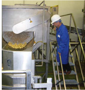
11 • Potato-peeling with roller peeler R-3012-100KK-S130. Screw diameter 1300, roller length 3000 mm.
