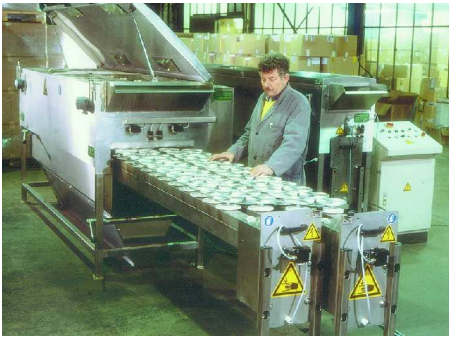
1 • Machine MSS-BM with two blade-peeling units, pulled out of the peeler.
