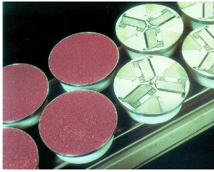
2 • Blade and carborundum discs combined here. Onion-peeling discs not shown.
