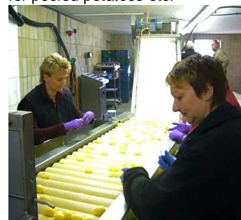
9 • Roller inspection table in a MSS peeling system.
