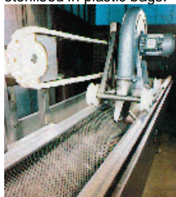
23 • Waste water technology: here separator with cleaning device.
