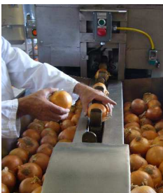
4 • Topping and tailing machine TT for onions.
