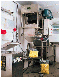
16 • Preserving & filling device, model 5-15; on the left a vacuum-packing machine.
