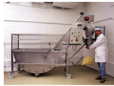
6 • Preserving and filling device BM 5-25 for peeled potatoes etc.
