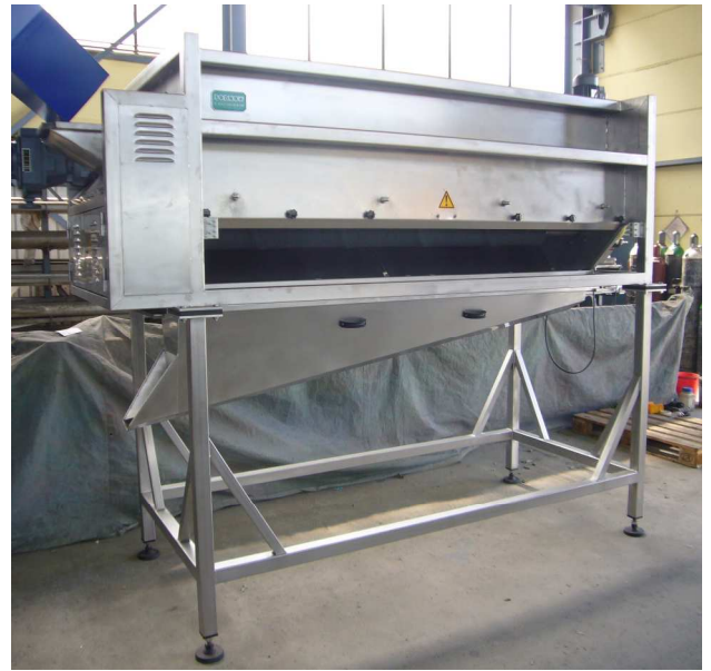
DORNOW roller peeling machine for higher capacities and more automatical lines
