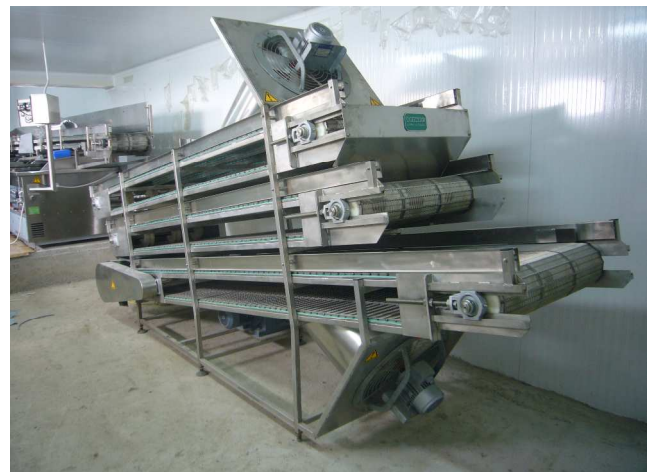
Cooling conveyor belt, open construction, capacity approx. 500 kg/h.
