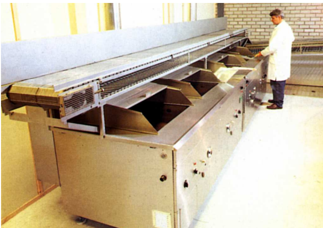
Overview: 2 Industrial fryers "Industry 300" with wire link belt on top
