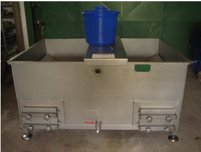
Storage bin for underwater storage and washing of cut French fries sticks
