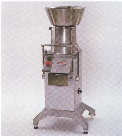
Hälde universal cutting machine for the slicing and dicing of tubers, roots and many types of vegetables.
