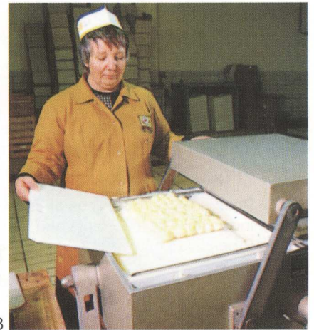
Vacuum-sealing device, available in various designs, also with gas-flushing facility.
