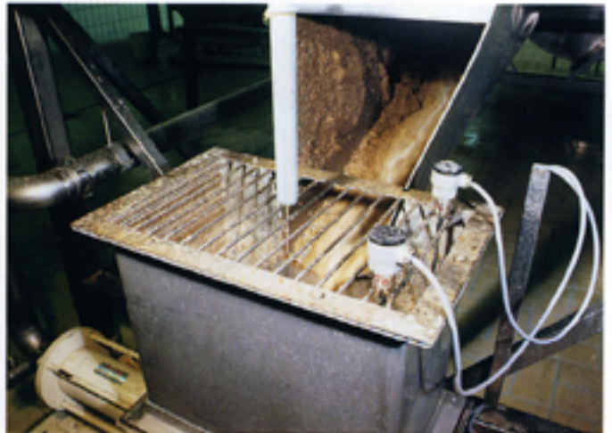
Potato waste peel, without the addition of water, flows into the collecting container of a pump.
