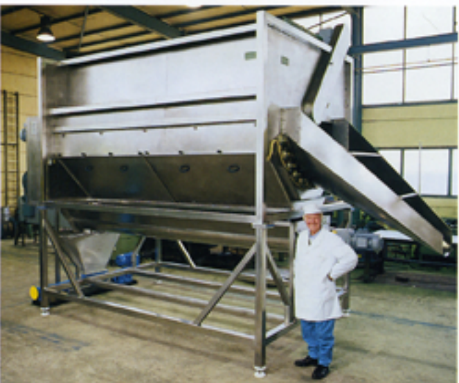
Roller peeling machine R-OW-150-A, internal diameter 1500 mm, for the peeling of celery roots, beetroot and carrots.
