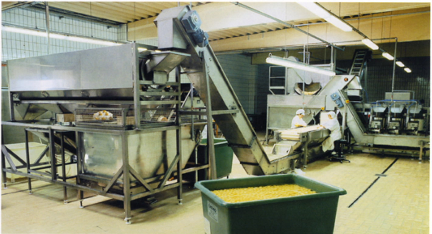
Complete peeling plant for potatoes in a ready-made meals factory: roller peeling machine R-OW-110, blade peeling line connected behind, roller inspection table, sorting system and halving and quartering machine.
