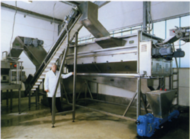
Roller peeling machine R-OW-60-A, internal diameter 600 mm, in an industrial potato peeling plant.
