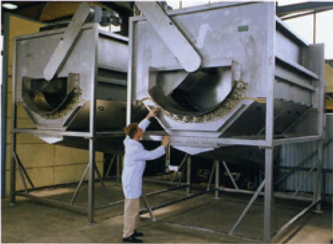
Two of the biggest roller peeling machines R-OW-150-A, internal diameter 1500 mm.
